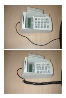
In the bottom picture, the cord has been replaced, this could allow capture of credit card data, if left unnoticed. Never allow direct physical access to the credit card device without owner/manager approval.
